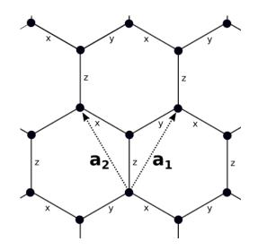
Figure 1: The honeycomb lattice with primitive vectors  $\mathbf{a}_1$  and  $\mathbf{a}_2$ , and x, y, and z-oriented links.
